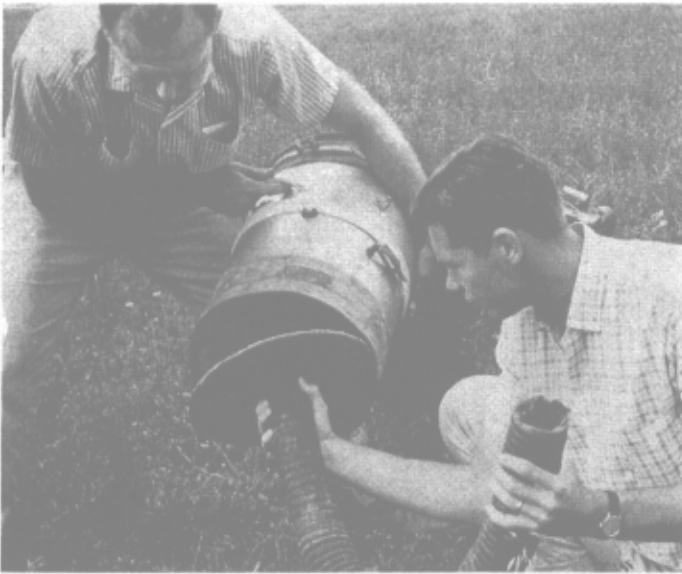
Placement of adapter hose for complete sampling.
